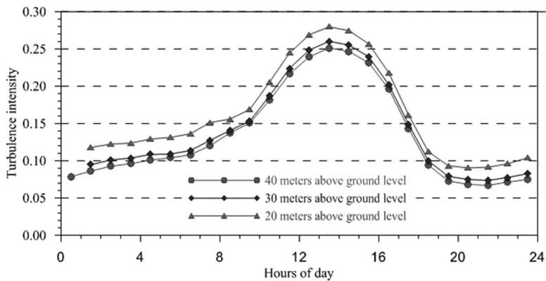
Figure 10 Diurnal variation of mean turbulence intensity at different heights.
