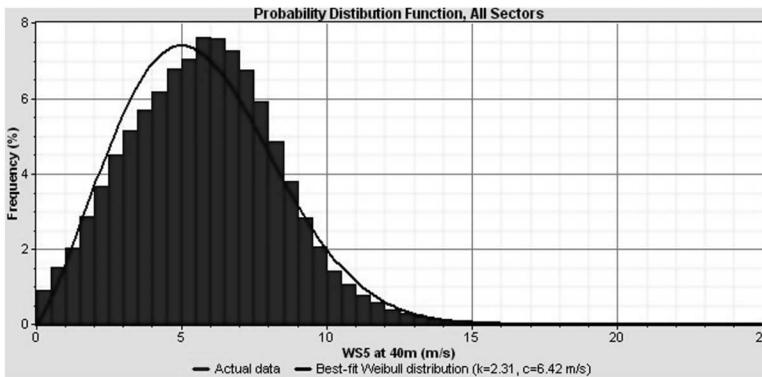
**Figure 5** Frequency distribution of wind speed at 40 meters above ground level during the period of October 2005 to October 2008.
