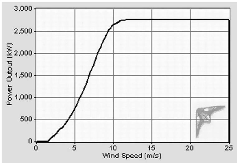
Figure 11 Wind power curve of V100 wind turbine from Vestas [24].
